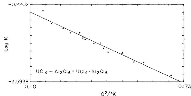
Figure 8.—Plot of  $\log K$  vs.  $1/T_{\text{min}}$  for reaction 20.
