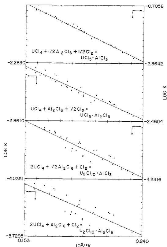
Figure 5.—Plots of  $\log K$  vs.  $1/T_{\min}$  for eq 9 using four different sets of  $n_1, n_2$ , and  $n_3$  values.
