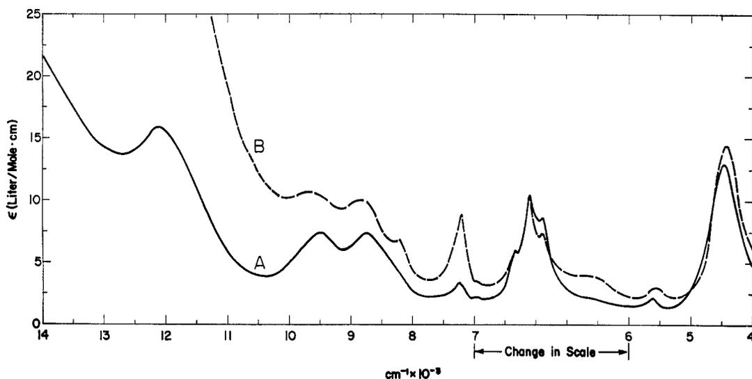
Figure 6.—“High-temperature” spectra of uranium pentachloride: A,  $\text{UCl}_4\text{-AlCl}_3\text{-Cl}_2$  system at 852°K; B,  $\text{UCl}_4\text{-Cl}_2$  system at 844°K.
