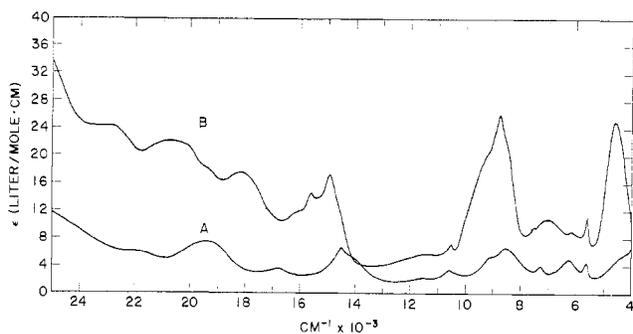
Figure 7.—Absorption spectra of gaseous  $\text{UCl}_4$  at  $1225^\circ\text{K}$  (A) and of gaseous  $\text{UCl}_2(\text{AlCl}_4)_2$  at  $845^\circ\text{K}$  (B).
