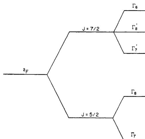
Figure 4.—Schematic energy level diagram for a  ${}^2F$  state split by the combined action of the spin-orbit coupling and octahedral ligand field perturbations.
