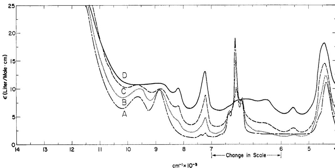
Figure 1.—Absorption spectra of gaseous uranium pentachloride at various temperatures: A, 597°K; B, 747°K; C, 844°K; D, 1031°K.
