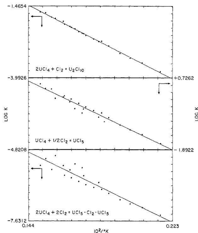
Figure 3.—Plots of  $\log K$  vs.  $1/T_{\text{min}}$  for reactions 3-5.
